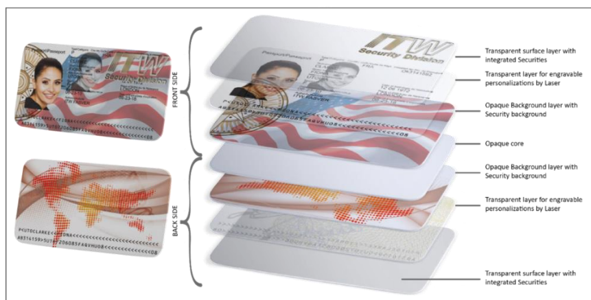
A typical Polycarbonate Card structure
