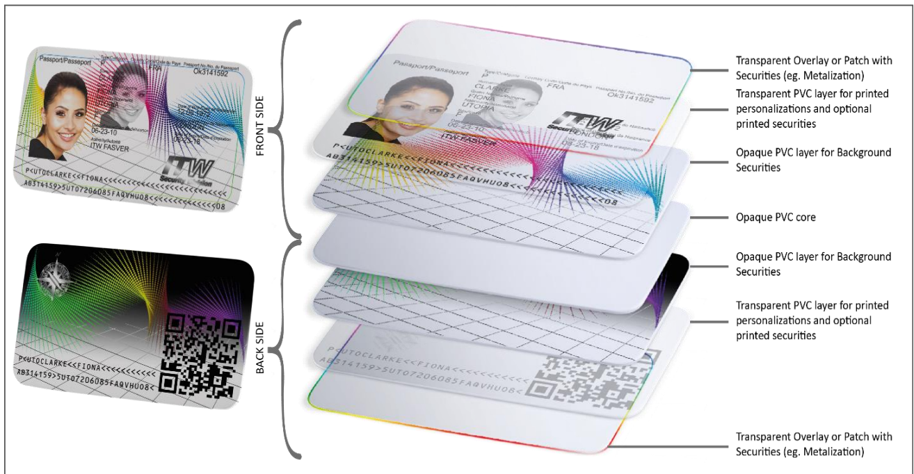
A typical PVC Card structure with multiple layers
